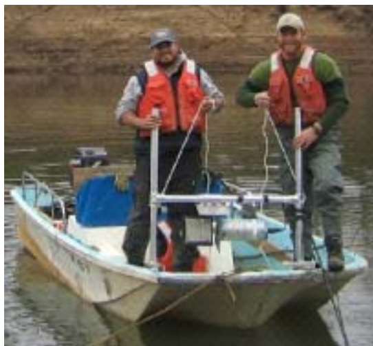
Technician Gery Cox and graduate student Warren Mitchell prepare to deploy a hydroacoustic transducer in the Roanoke River to estimate run size of several anadromous species.
